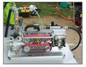
**Plumett Mini Jet Blowing / Jetting machine**
