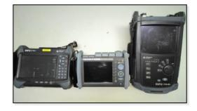
**Optical Time Domain Reflectometer** (OTDR)
